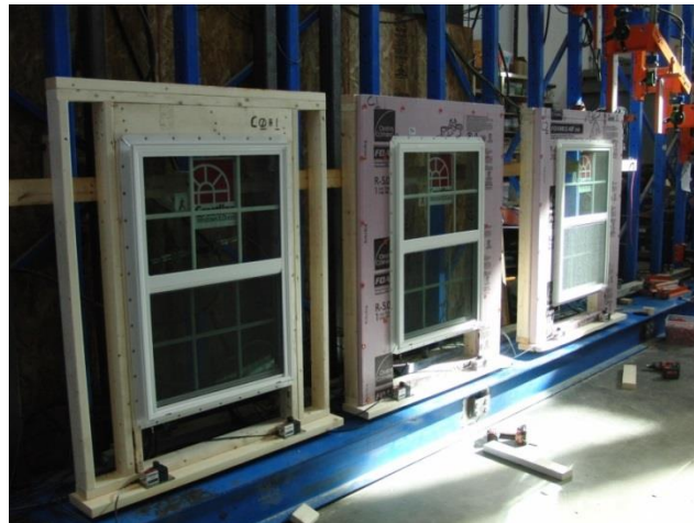
Photo 1: Long-Term Deflection Under Self-Weight Testing
