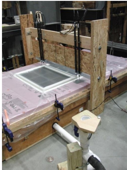
Photo 3: Wind Pressure Loading Test Setup
