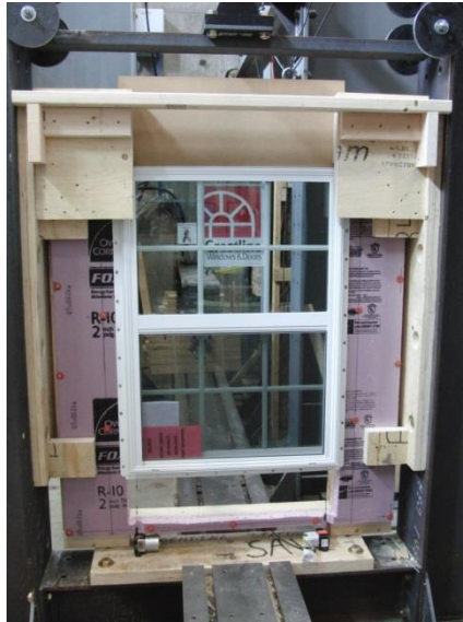
Photo 2: Structural Loading – Fastener/Flange Capacity
